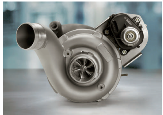
Figure 2.213 Waste gate actuator under electronic control. (Source: Bosch Media)
